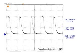
500kHz Frequency, 125 Amps Output
