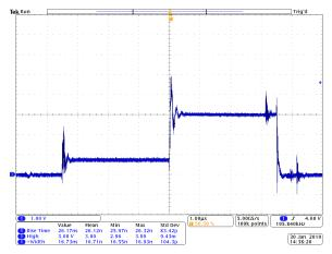
Internal trigger: 100 kHz, 3.5  $\mu$ s bias and 3.5  $\mu$ s main pulse width, 1 A bias current, 3 A main current.
