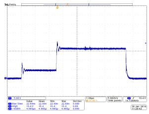
Internal trigger: 100 kHz, 2.5 μs bias and 5.0 μs main pulse width, 6 A bias current, 16 A main current.
