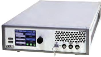
The PCX-7420 provides both QCW (pulsed), and CW (DC) outputs. It can drive a bias current from 0.050 A to 5.8 A, and pulsed/QCW currents from 3 A to 21.5 A. A new feature allows the bias current to be pulsed and triggered independent of the main current trigger.
