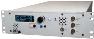
The PCX-7420 B is an air-cooled, high-powered CW/QCW current source designed to drive diode lasers, bars, and arrays. It can drive a bias current from 0.050 A to 5.8 A (can be triggered independently of the primary current pulse). The pulsed output current is adjustable from 3.0 A to 21.5 A.
