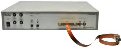
Designed for precision pulsing of semiconductor devices for pulsed I-V characterization, provides fast rise and fall times with minimal overshoot, undershoot, and ringing, and fast settling times. The controlled-voltage waveform allows the device under test (DUT) to stabilize at voltage within a few hundred nanoseconds, allowing I-V measurements to be made before device heating begins.
