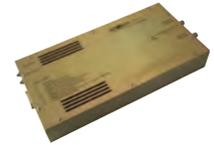
Typical applications are instrument calibration, component testing, beam steering as well as photo multiplier tube (PMT) and microchannel plate (MCP) gating. The PVM-1001 can achieve zero to 950 V in less than 10 ns (Rise Time). This adjustable pulsed voltage source is capable of providing pulse widths from 55 ns to 10,000 ns with a standard frequency range up to 1 MHz. The PVM-1001 can also provide a 5 MHz burst. The module is designed for a 50 ohm resistive load.
