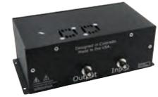
Typical applications are instrument calibration, component testing as well as photo multiplier tube (PMT) and microchannel plate (MCP) gating. The PVM-1001 can achieve zero to -950 V in less than 10 ns (Rise Time). This adjustable pulsed voltage source is capable of providing pulse widths from 55 ns to 10,000 ns with a standard frequency range up to 1 MHz. The PVM-1001 can also provide a 5 MHz burst. The module is designed for a 50 ohm resistive load.
