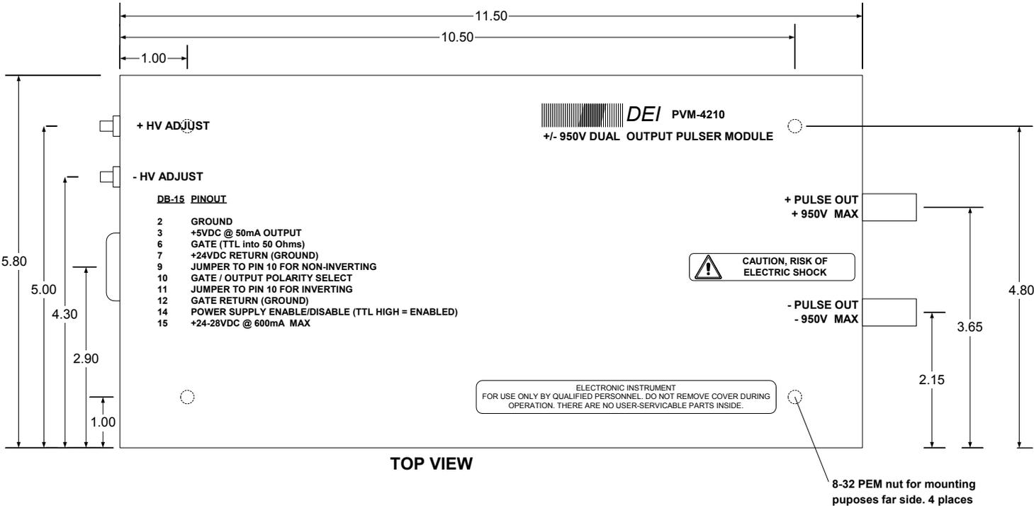
*PVM-4210 Mechanical Dimensions And Mounting Hole/Connector Locations
