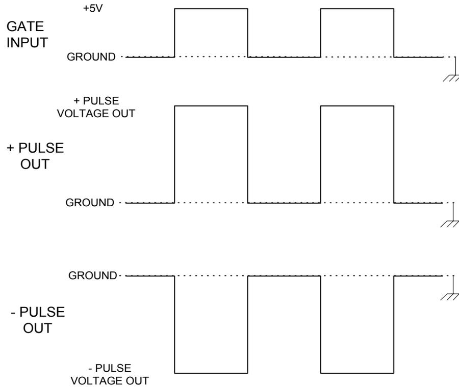
***Output Pulse Configuration With Non-Inverted Gate Selected***
