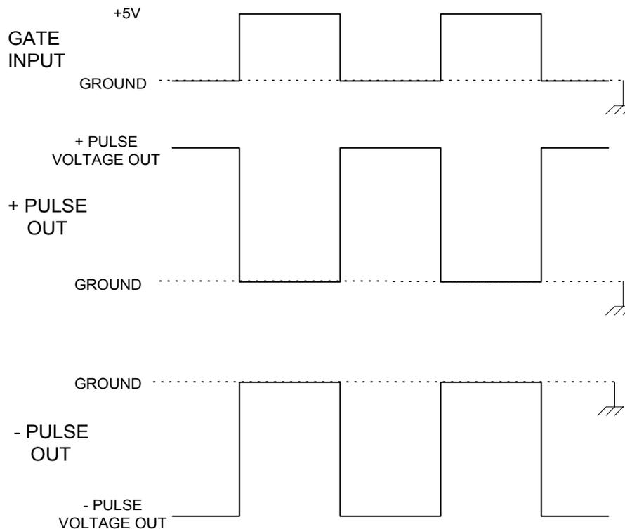
***Output Pulse Configuration With Inverted Gate Selected***
