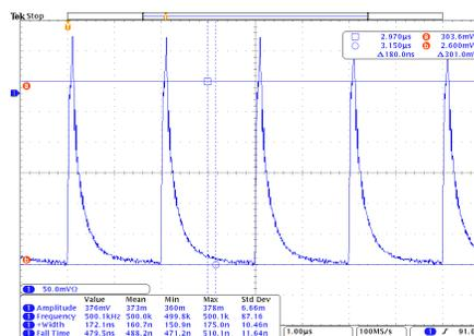
500 KHz, 172 ns Pulse Width, 60 A Output
