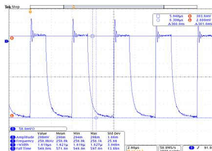
250 kHz, 1.6  $\mu$ s Pulse Width, 60 A Output
