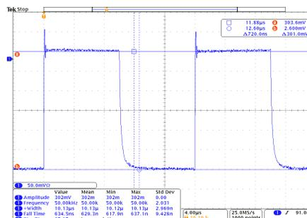
50 kHz, 10  $\mu$ s Pulse Width, 60 A Output
