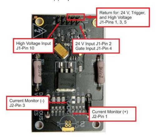
The gate signal should be connected to pin 4 of J1. The shield of the coaxial cable should be connected to any one of the Return pins (1, 3, or 5) of connector J1. To improve pulse fidelity, all connections should be as short as possible. The gate signal should be TTL (+3V to +5V) into  $50\Omega$ . The voltage level of the pulse generator should be set while terminated into a  $50\Omega$  termination (such as the  $50\Omega$  input of an oscilloscope) prior to connection to the PCO-7114.
